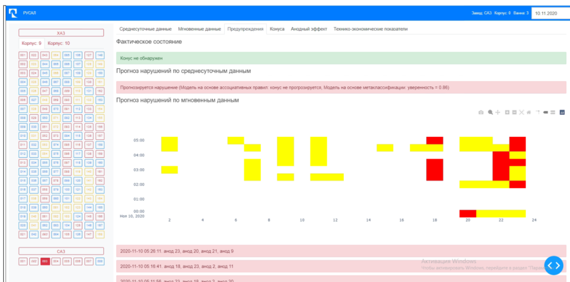
Figure 7. Example of indication of irregularities and information messages on the occurrence of disruptions. Yellow markers: anodes with “development of process disruptions”, Red markers: anodes with “occurrence of process disruptions”.
