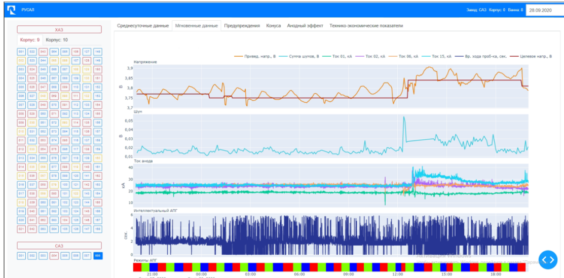
Figure 6. Example of instant monitoring parameters. Top row: voltage (V), 2 nd row: cell noise, [mV], 3 rd row: anode current, [kA], Bottom row: operating modes of Al 2 O 3 point feeding system, [-].
